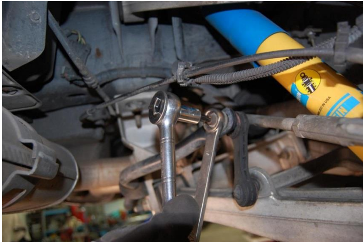
An 18mm wrench is used to turn the nut while a T40 Torx bit holds the stud. Of course you can spin the stud on the old pieces for removal.
