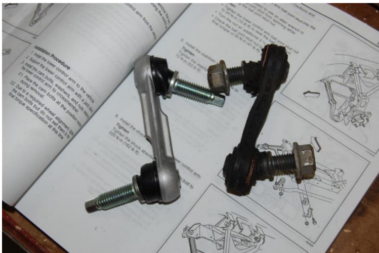
You can see the difference in this original 1999 anti-roll bar end link which has some distortion from age. The aluminum end links available from Corvette Central are stout pieces with new rubber seals.
