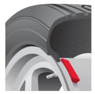
TPMS can come in one of two types: *direct* or *indirect*. Each type of system uses different mechanical setups and methods to monitor pressure and alert you when pressure is low. Direct TPMS measures air pressure through dedicated sensors in the wheel, while indirect TPMS estimates low pressure based on tire rotation speed.
