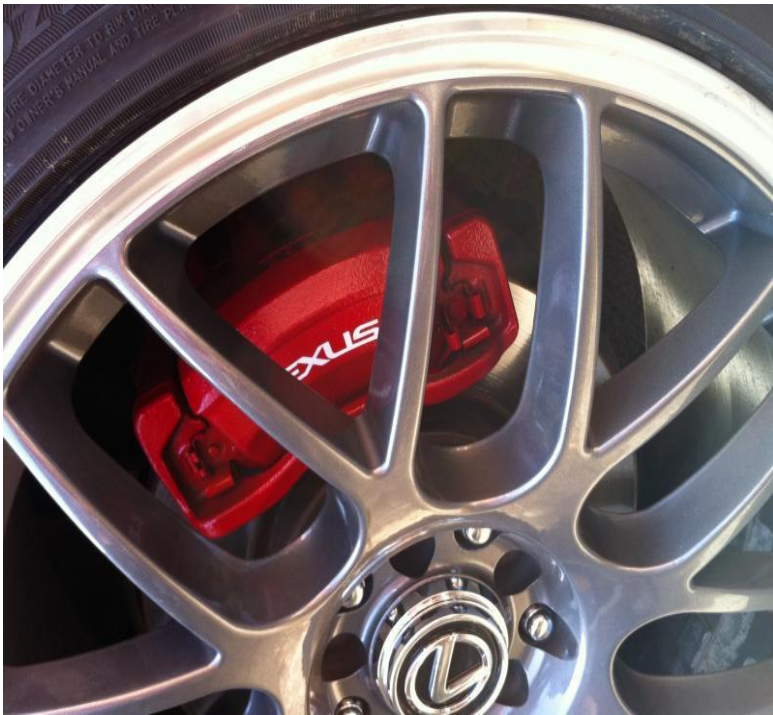
Figure 2. Check along the outside bead of the wheel to see if there are any bends or damage.
