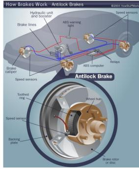
A one-channel, one-sensor scheme is easy to identify. Usually there will be one brake line going through a T-fitting to both rear wheels. The speed sensor can be located by looking for an electrical connection near the differential on the rear-axle housing.
