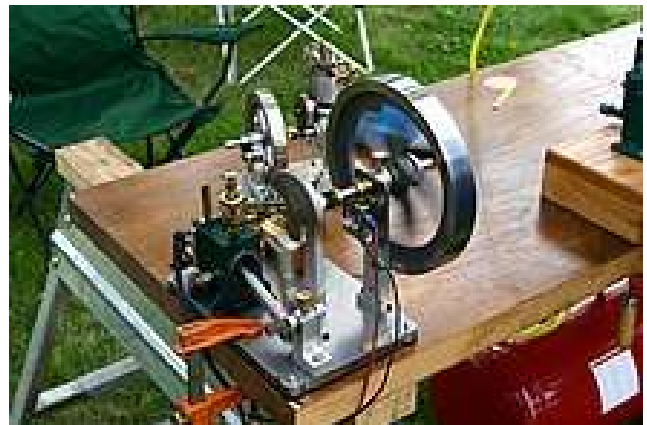
A small engine with Atkinson-style linkages between the piston and flywheel. Modern Atkinson-cycle engines do away with this complex energy path.
